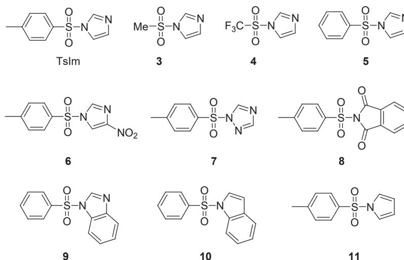
**Fig. 1** Structures of analogues of TsIm tested as coupling reagents.
