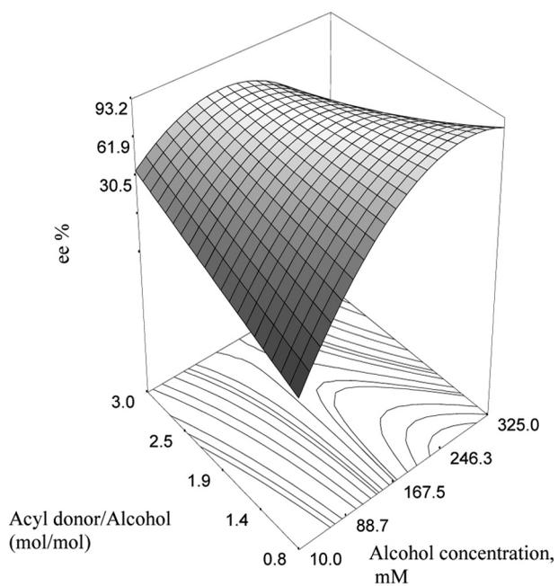
**FIGURE 2** Response surface plot showing the mutual effect of acyl donor/alcohol (mol/mol) and alcohol concentration when the other variables are held at zero level.
