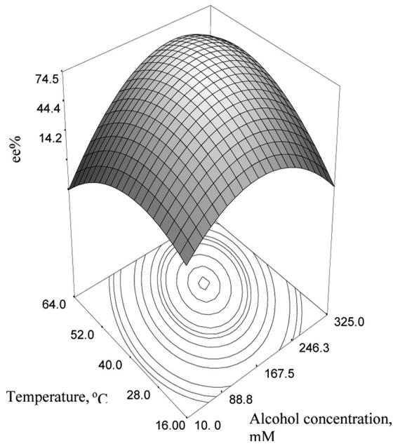
**FIGURE 4** Response surface plot showing the mutual effect of temperature and alcohol concentration when the other variables are held at zero level.
