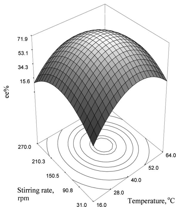
**FIGURE 6** Response surface plot showing the mutual effect of stirring rate and temperature when the other variables are held at zero level.
