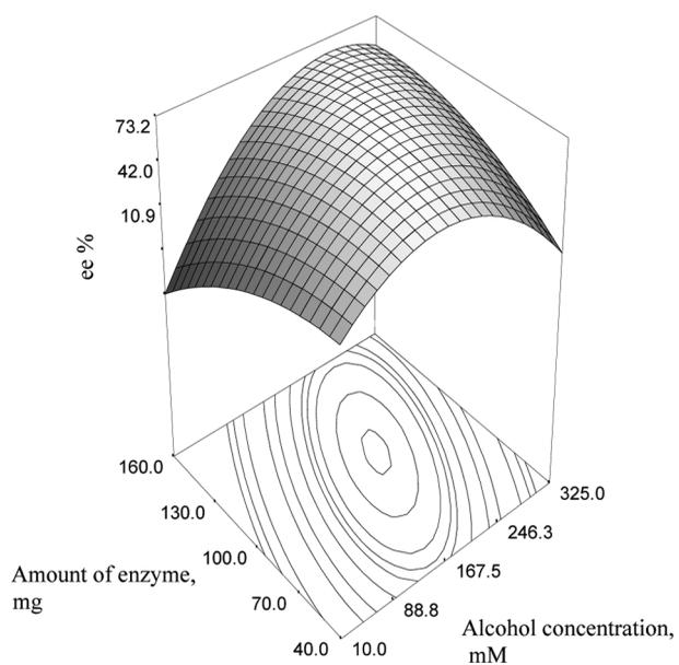
**FIGURE 3** Response surface plot showing the mutual effect of amount of enzyme and alcohol concentration when the other variables are held at zero level.
