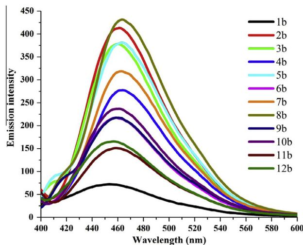
**Fig. 4.** The emission spectra of 1-(3,4-dimethylphenyl)-3-(4-fluorophenyl)-5-(4-alkoxyphenyl)-2-pyrazolines (**1b–12b**) in DMF–H<sub>2</sub>O (3:7) system at concentration of  $1 \times 10^{-7}$  mol L<sup>-1</sup>.
