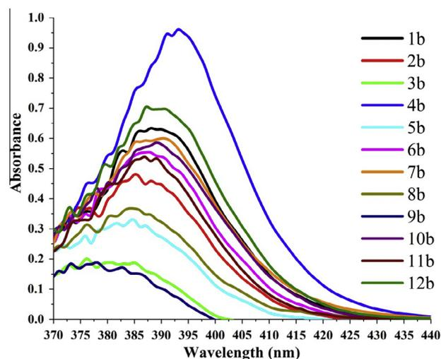
**Fig. 3.** The UV–Vis absorption spectra of 1-(3,4-dimethylphenyl)-3-(4-fluorophenyl)-5-(4-alkoxyphenyl)-2-pyrazolines (**1b–12b**) in DMF–H<sub>2</sub>O (3:7) system with the concentration of  $1 \times 10^{-5}$  mol L<sup>-1</sup>.
