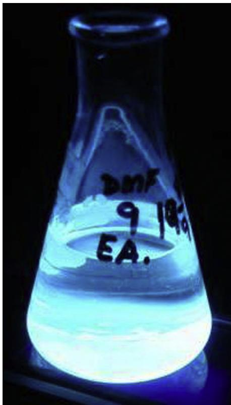
**Fig. 7.** Photoluminescence of 1-(3,4-dimethylphenyl)-3-(4-fluorophenyl)-5-(4-nonyloxyphenyl)-2-pyrazoline (**9b**) in ethyl ethanoate at  $1 \times 10^{-3}$  mol L<sup>-1</sup> concentration.
