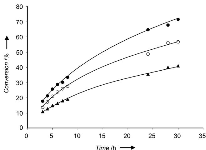
**Figure 1.** Cellulose conversion without (▲) and with the catalysts Pt/AIW (●) and AIW (○) as a function of time.
