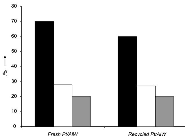
Figure 5. Recycling experiment with Pt/AIW (black: conversion; white: acetol yield; grey: propylene glycol yield). Conditions: cellulose (1.6 g), catalyst (0.65 g), water (65 mL), 5 MPa H<sub>2</sub>, 190 °C, 24 h.
