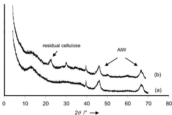
Figure 4. XRD spectra of Pt/AIW (a) before and (b) after reaction.
