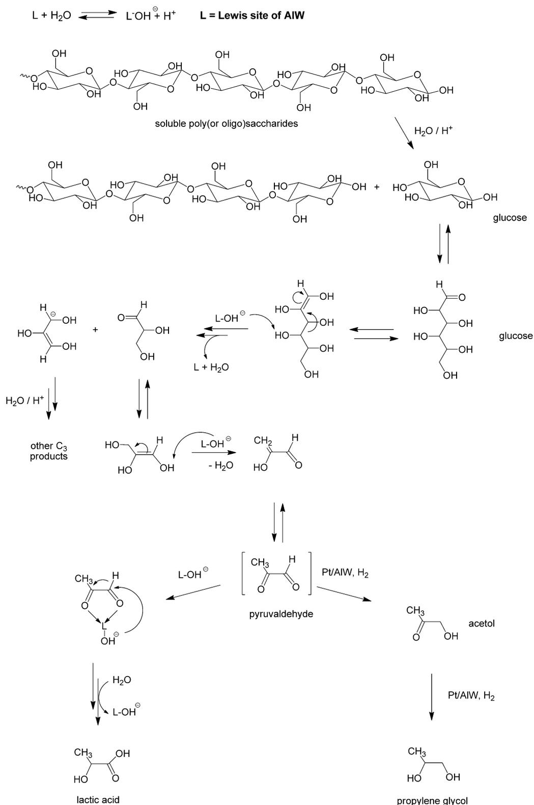
**Scheme 1.** Proposed mechanism for the formation of lactic acid, acetol and propylene glycol from cellulose with AIW or Pt/AIW catalysts under H<sub>2</sub>.
