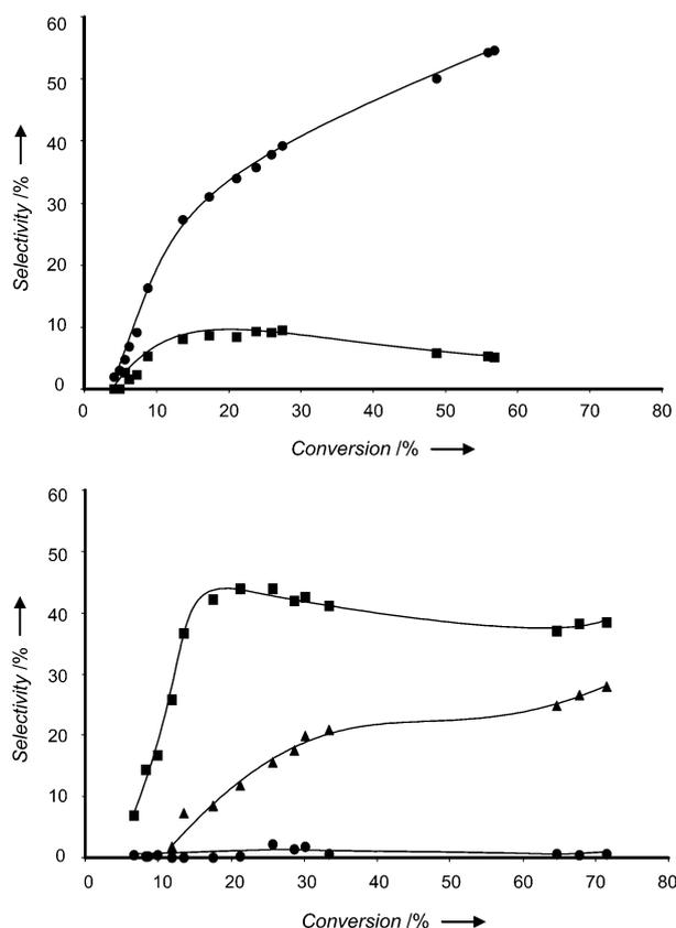
**Figure 3.** Evolution of the selectivities (● lactic acid; ■ acetol; ▲ propylene glycol) as a function of cellulose conversion with AIW (top) and Pt/AIW (bottom).
