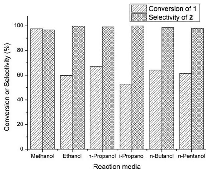
Fig. 2. Influence of solvent in oxidative C—C bond cleavage reaction (0.20 g of **1**, 0.05 g NiO<sub>x</sub>, 20 mL solvent, under 0.3 Mpa of O<sub>2</sub>, at 140 °C, for 3 h).
