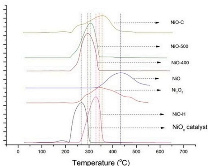
Fig. 1. The  $H_2$ -TPR detection of nickel oxides prepared using different methods.
