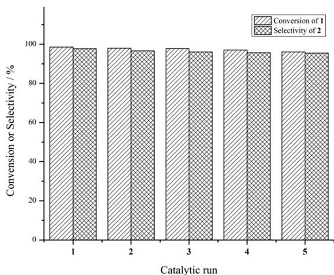
Fig. 3. Recycling of NiO<sub>x</sub> on the oxidative C—C bond cleavage of **1** Reaction conditions: 0.20 g of **1**, 0.05 g catalyst, 0.005 g K<sub>2</sub>CO<sub>3</sub>, in 20 mL methanol, under 0.3 Mpa of O<sub>2</sub>, at 140 °C, for 3 h).
