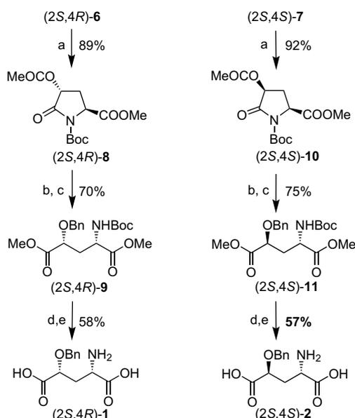
Scheme 2. (a) RuO<sub>2</sub>·xH<sub>2</sub>O, NaIO<sub>4</sub>, H<sub>2</sub>O, AcOEt; (b) PS-CO<sub>3</sub>, MeOH; (c) Ag<sub>2</sub>O, PhCH<sub>2</sub>Br, Et<sub>2</sub>O; (d) NaOH, MeOH; (e) 30% CF<sub>3</sub>COOH/CH<sub>2</sub>Cl<sub>2</sub>.
