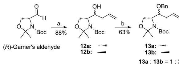
Scheme 3. (a) CH<sub>2</sub>=CHCH<sub>2</sub>MgCl, ZnCl<sub>2</sub>, THF; (b) BnBr, NaH 60%, THF.
