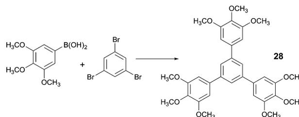
**Scheme 2** General conditions: 3,4,5-trimethoxyphenylboronic acid, 1,3,5-tribromobenzene, K<sub>2</sub>CO<sub>3</sub>, Pd(PPh<sub>3</sub>)<sub>4</sub>, MW (250 W, 115 °C) in dioxane : water (5 : 1) for 35 min.
