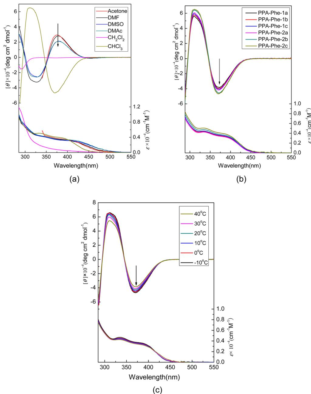
**Figure 2.** CD (upper) and UV-vis (lower) spectra of (a) PPA-Phe-2c in variable solvents at 25 °C, (b) PPA-Phe-1a-c and PPA-Phe-2a-c in CHCl<sub>3</sub> at 25 °C, and (c) PPA-Phe-1a in CHCl<sub>3</sub> at different temperature ( $c = 1$  mg/mL).
