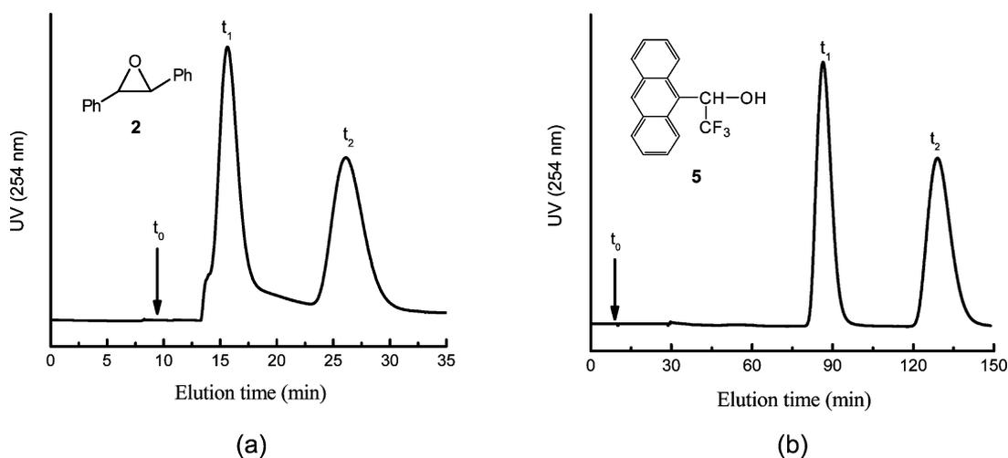
**Figure 5.** Chromatograms for the resolution of (a) *trans*-stilbene oxide (2) on PPA-Phe-2c and (b) 1-(9-anthryl)-2,2,2-trifluoroethanol (5) on PPA-Phe-1a with hexane/2-propanol (95/5) as eluent.
