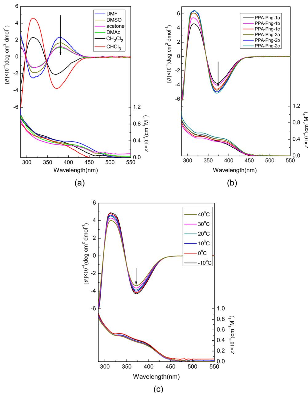
**Figure 3.** CD (upper) and UV-vis (lower) spectra of (a) PPA-Phg-1a in variable solvents at 25 °C, (b) PPA-Phg-1a-c and PPA-Phg-2a-c in CHCl<sub>3</sub> at 25 °C, and (c) PPA-Phg-1a in CHCl<sub>3</sub> at different temperature ( $c = 1$  mg/mL).
