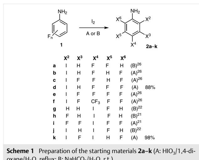
**Scheme 1** Preparation of the starting materials **2a–k** (A: HIO<sub>3</sub>/1,4-dioxane/H<sub>2</sub>O, reflux; B: NaHCO<sub>3</sub>/H<sub>2</sub>O, r.t.)
