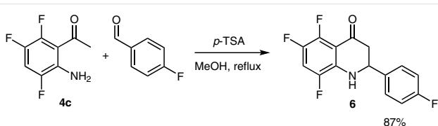
**Scheme 5** Preparation of 5,6,8-trifluoro-2-(4-fluorophenyl)-2,3-dihydroquinolin-4(1*H*)-one (**6**)
