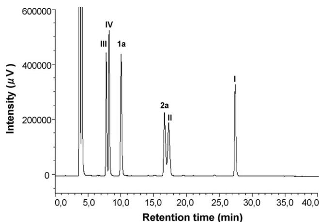
Fig. 7. A typical RP-HPLC chromatogram of a mixture of the four candidates for internal standards (compounds I–IV), together with two of the  $\Delta^5$ -bile acid conjugates (1a and 2a) identified from the urine of a patient with NP-C1.
