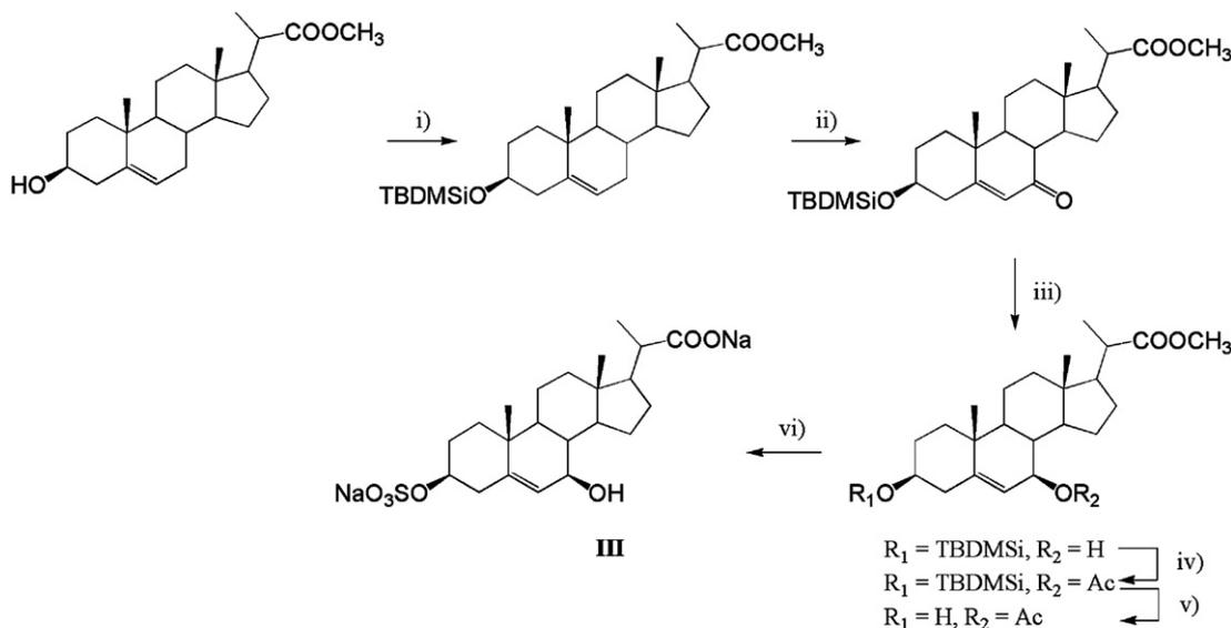
**Reagents and Conditions:** i) TBDMSiCl, imidazole, py., DMF, r.t., 1.5h. ii) PDC, *t*-BHPPO, benzene, r.t., 24h. iii) Zn(BH<sub>4</sub>)<sub>2</sub>, ether, r.t., 2h. iv) Ac<sub>2</sub>O, py., r.t., 3h. v) 10%-HCl, MeOH, acetone, r.t., 15min. vi) SO<sub>3</sub><sup>-</sup>N<sup>+</sup>(CH<sub>3</sub>)<sub>3</sub>, py., r.t., 1h, and then 1M NaOH/MeOH, reflux, 8h.
