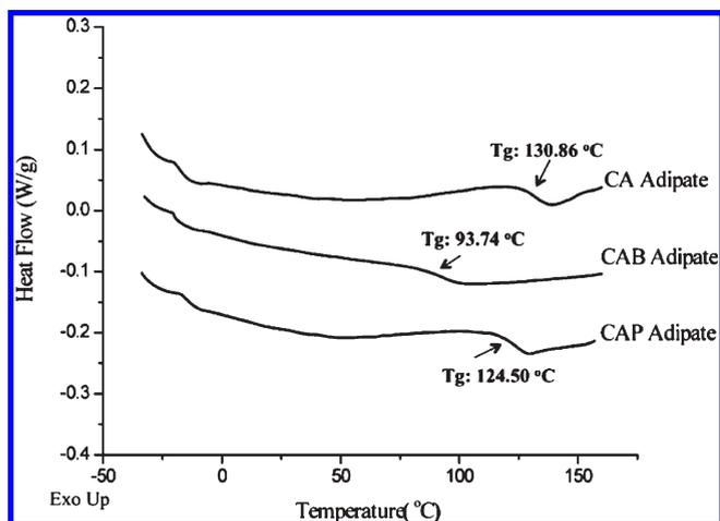
Figure 6. DSC curves of cellulose adipate derivatives at heating rate 10 °C/min (2nd heat).
