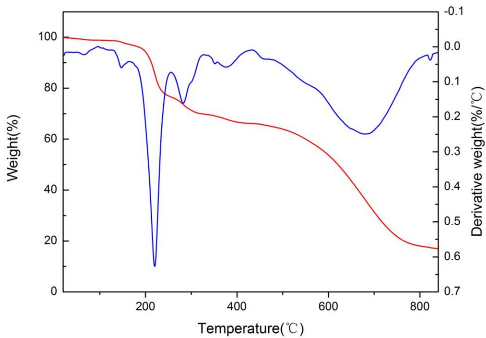
**Figure 1.** TGA/DTG curve of HDHPCP
