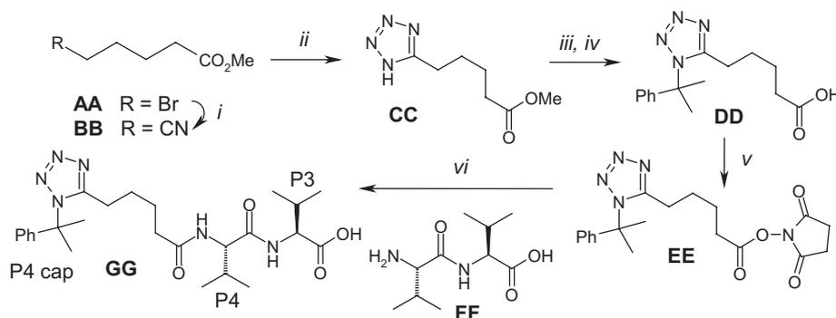
**Scheme 1.** Synthesis of P4 tetrazole capped dipeptidyl acid GG. Reagents and conditions: (i) KCN/aq EtOH, 74%; (ii)  $\text{NaN}_3/\text{Et}_3\text{NHCl}$ , 68%; (iii)  $\text{Ph(Me)=CH}_2/\text{Cl}_3\text{CCO}_2\text{H}$ , 95%; (iv) aq NaOH, 75%; (v) HOSu/EDCI/DIEA, 75%; (vi) **FF**/DIEA, 91%.
