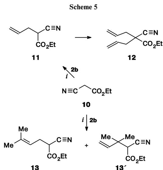
*i.* Pd(dba)<sub>2</sub>, ligand, K<sub>2</sub>CO<sub>3</sub>, DMF 20 °C.
