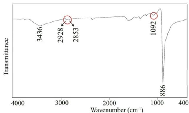
FIGURE 4 FTIR spectrum of the  $\text{Ag}_2\text{Cr}_2\text{O}_7$  NPs
