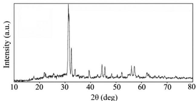
FIGURE 5 XRD spectra of the  $\text{Ag}_2\text{Cr}_2\text{O}_7$  NPs
