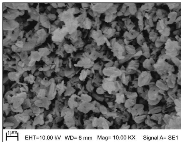
**FIGURE 2** SEM images of the  $\text{Ag}_2\text{Cr}_2\text{O}_7$  NPs
