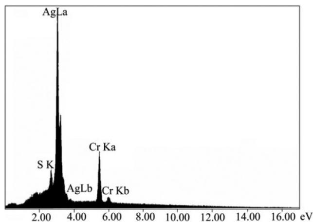
FIGURE 3 EDS analysis of the  $\text{Ag}_2\text{Cr}_2\text{O}_7$  NPs
