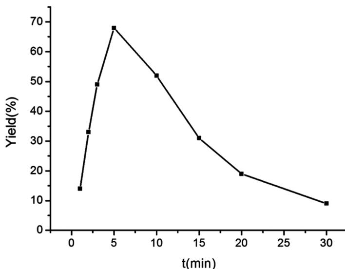
**Figure 3.** Effect of residence time on the yield of the reaction of ester-substituted aniline. Temperature: 120°C; pressure: 75 psi.
