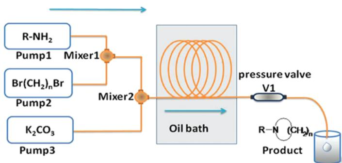
**Abstract** A practical, rapid, and efficient reaction using microreactors for the direct N-alkylation from aniline derivatives and alkyl dihalides has been achieved in the presence of aqueous potassium carbonate at an elevated temperature. This improved synthetic methodology provides a straightforward microfluid approach to the synthesis of a variety of N-aryl azacycloalkanes.
