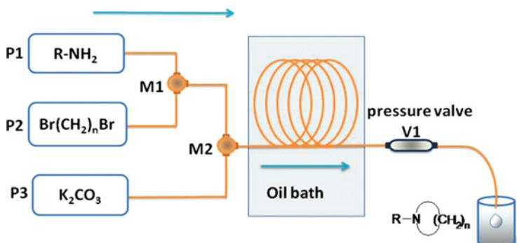
**Figure 1.** Microflow system consisting of three injection pumps (P1, P2, P3), two T-shaped micromixers (M1, M2), and one peek microtube reactor (inner diameter  $\phi = 0.5$  mm, length  $L = 200$  cm). (Figure is provided in color online.)
