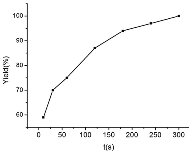
**Figure 2.** Effect of residence time on the yield of the reaction of substrate aniline at fixed temperature and pressure. The yield detected by HPLC; temperature: 20°C; pressure: 75 psi.
