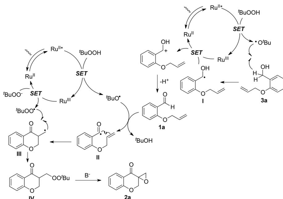
**Scheme 3.** Proposed mechanism of the present tandem catalysis
