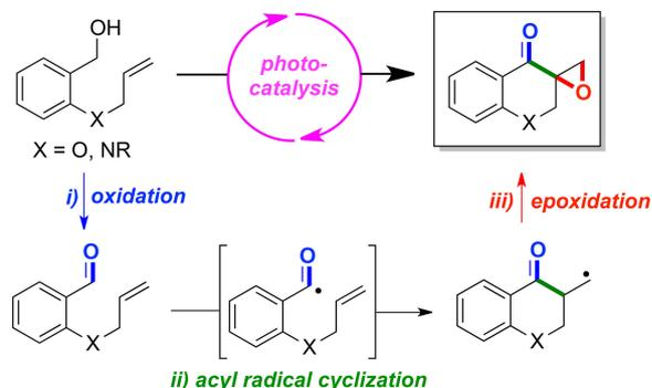
**Scheme 1.** Synthetic approach to the spiroepoxy chroman-4-ones and their nitrogen-containing derivatives via a visible light-induced tandem oxidation/radical cyclization/epoxidation sequence.
