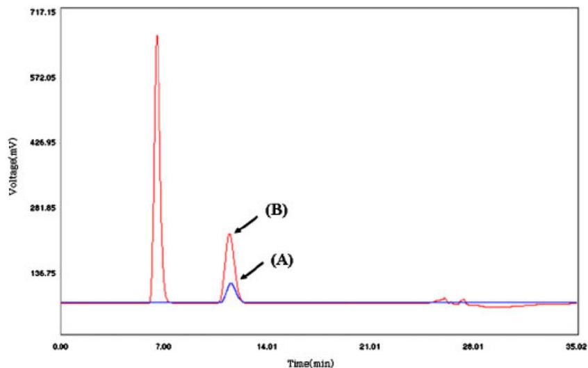
**Figure 3.** HPLC chromatograms of co-injection of purified  $^{125}\text{I}$ -labelled compound **1** (A;  $\gamma$ -radioactivity detector) and standard compound (B; UV detector). (Waters; deltapack RP-18,  $10\ \mu\text{m}$ ,  $7.9 \times 250\ \text{mm}$ , EtOH/H<sub>2</sub>O = 5:95 (v/v), flow rate: 2.0 ml/min, retention time: 10.9–12.3 min).
