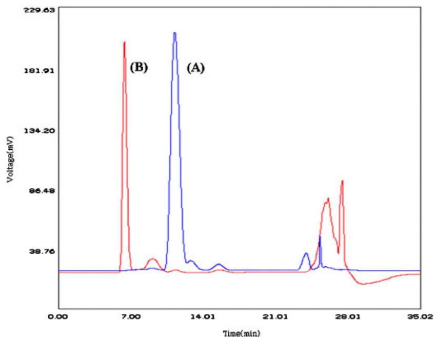
**Figure 2.** HPLC chromatograms of purified  $^{125}\text{I}$ -labelled compound **1** by  $\gamma$ -radioactivity detector (A) and ascorbic acid (additive for radioprotection) at 254 nm by UV detector (B) (Waters; deltapack RP-18,  $10\ \mu\text{m}$ ,  $7.9 \times 250\ \text{mm}$ , EtOH/H<sub>2</sub>O = 5:95 (v/v), flow rate: 2.0 ml/min, retention time of compound **1**: 10.9–12.3 min).
