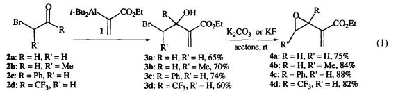
We avoided aqueous alkaline conditions for the epoxidation of these bromohydrins due to the presence of the ester moiety. We conducted the cyclizations in dry acetone and obtained 75–88% yields of the vinylepoxides. The epoxidation of **3a–c** was successfully carried out with  $K_2CO_3$  as base (Eq. 1). However, the trifluoromethyl bromohydrin **3d** afforded only 65% yield of the corresponding epoxide **4d**, and we improved the yield to 82% by replacing  $K_2CO_3$  with KF.<sup>6</sup>
