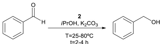
Fig. 3. TH of benzaldehyde with *i*PrOH/K<sub>2</sub>CO<sub>3</sub> using complex 2.
