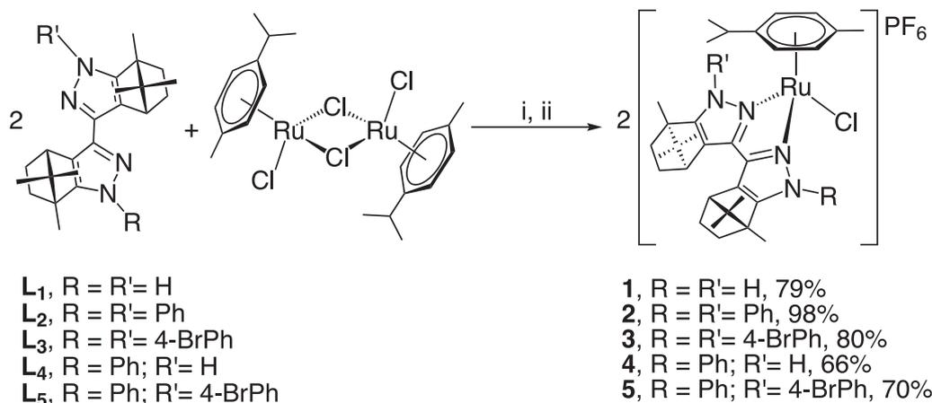
**Scheme 2.** Synthesis of ruthenium (II) complexes 1–5 with  $C_2$  and  $C_1$  (+)-camphopyrazole ligands. i)  $\text{CHCl}_3$  or  $\text{CH}_2\text{Cl}_2$ , room temperature, 24 h. ii) Ethanol,  $\text{NH}_4\text{PF}_6$ , room temperature, 24 h.
