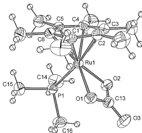
Figure 2. ORTEP drawing of **2d**· $\text{H}_2\text{O}$  showing 50% probability thermal ellipsoids. The  $\text{H}_2\text{O}$  molecule has been omitted for clarity. Selected bond lengths [Å] and angles [°]: Ru1–O1 2.104(2), Ru1–O2 2.091(2), O1–C13 1.325(4), O2–C13 1.315(4), O3–C13 1.239(4), Ru1–P1 2.343(1); O1–Ru1–O2 62.81(8), C13–O1–Ru1 92.2(2), C13–O2–Ru1 93.1(2), O1–C13–O2 111.8(2), O1–C13–O3 123.7(3), O2–C13–O3 124.5(3), O1–Ru1–P1 88.61(7), O2–Ru1–P1 84.25(7).
