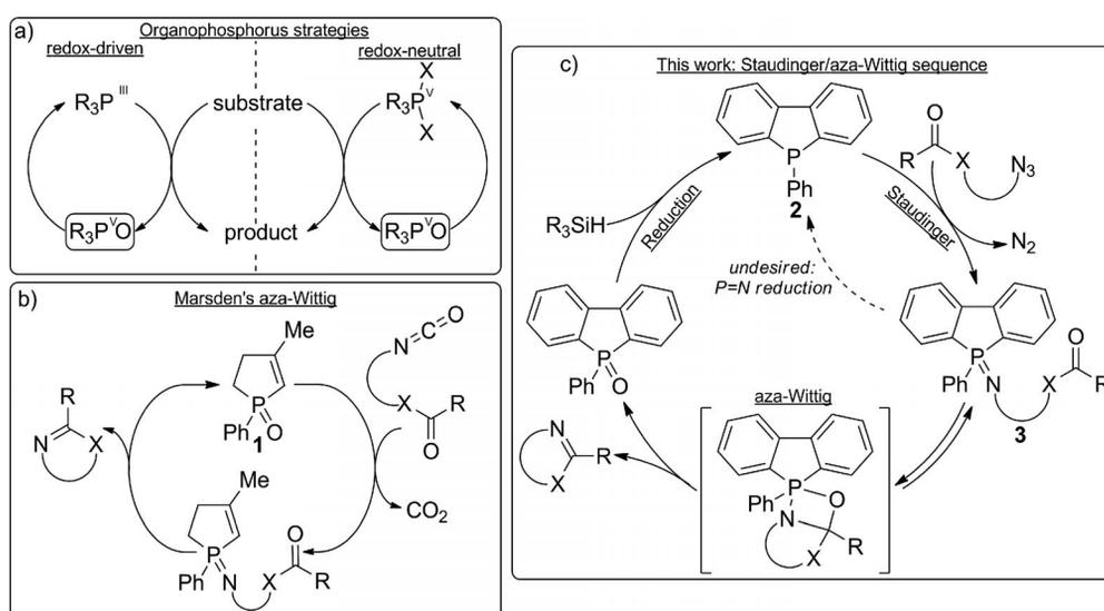
Scheme 1. a) Organophosphorus strategies by either redox-driven or redox neutral strategies; b) the aza-Wittig as developed by Marsden et al. via the redox neutral reaction pathway; c) the proposed mechanistic cycle for the Staudinger/aza-Wittig sequence as presented in this paper.
