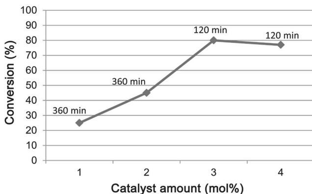
**Fig. 2** Optimization of the catalyst amount in synthesis of **4a** at 80 °C under solvent-free conditions
