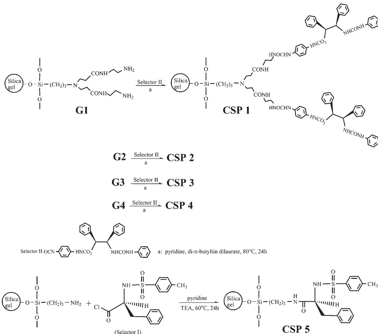
Fig. 1. The synthetic scheme of CSPs 1-5.
