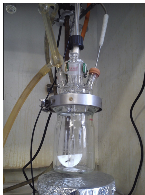
Fig. 1. Suspension polymerization reactor used in this study.
