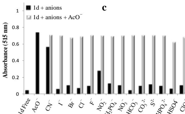
**Fig. 5.** a) UV-Vis absorption spectra of **1d** ( $3 \times 10^{-5}$  M) in the presence of 10 equiv. of various anions in DMSO/ $\text{H}_2\text{O}$  (9/1). Effect of competitive anions (10 equiv.) on the interaction of; b) **1d**/ $\text{CN}^-$  (10 equiv.) and c) **1d**/ $\text{AcO}^-$  (10 equiv.)
