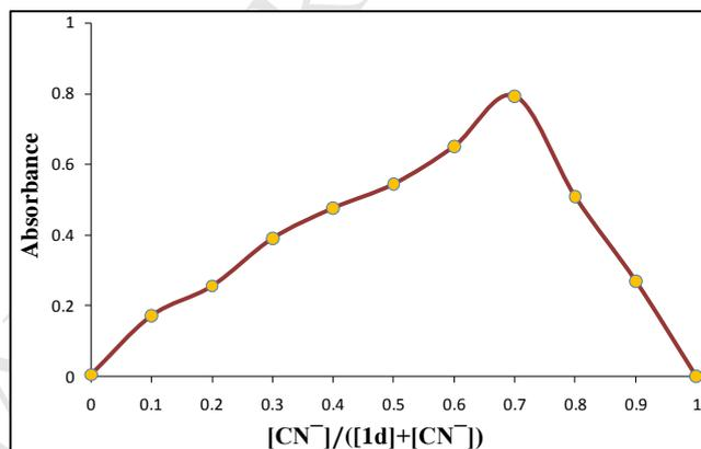
**Fig. 9.** Job's plot for stoichiometry of binding between receptor **1d** with  $\text{CN}^-$  in  $\text{DMSO}/\text{H}_2\text{O}$  (9/1) ( $\lambda = 591$  nm)
