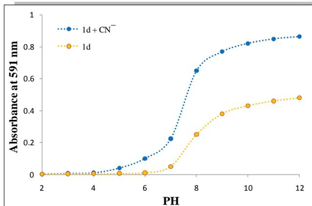
**Fig. 6.** Effect of pH on the UV-Vis spectra of sensor **1d** ( $3 \times 10^{-5}$  M) and **1d** containing  $\text{CN}^-$  ion at 591 nm
