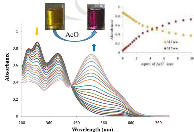
**Fig. 8.** UV-Vis absorption spectra of sensor **1d** ( $3 \times 10^{-5}$  M in  $\text{DMSO}/\text{H}_2\text{O}$  (9/1)) upon addition of  $\text{AcO}^-$  (0-10 equiv.). Inset showing the binding isotherm at selected wavelengths
