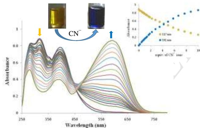
**Fig. 7.** UV-Vis absorption spectra of sensor **1d** ( $3 \times 10^{-5}$  M in  $\text{DMSO}/\text{H}_2\text{O}$  (9/1)) upon addition of  $\text{CN}^-$  (0-10 equiv.). Inset showing the binding isotherm at selected wavelengths
