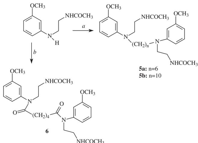
Scheme 2. Reagents and conditions: (a)  $\text{Br}(\text{CH}_2)_n\text{Br}$ ,  $\text{K}_2\text{CO}_3$ ,  $\text{DMF}$ ,  $100\text{ }^\circ\text{C}$ ; (b) adipoyl chloride,  $\text{TEA}$ ,  $\text{THF}$ , rt.
