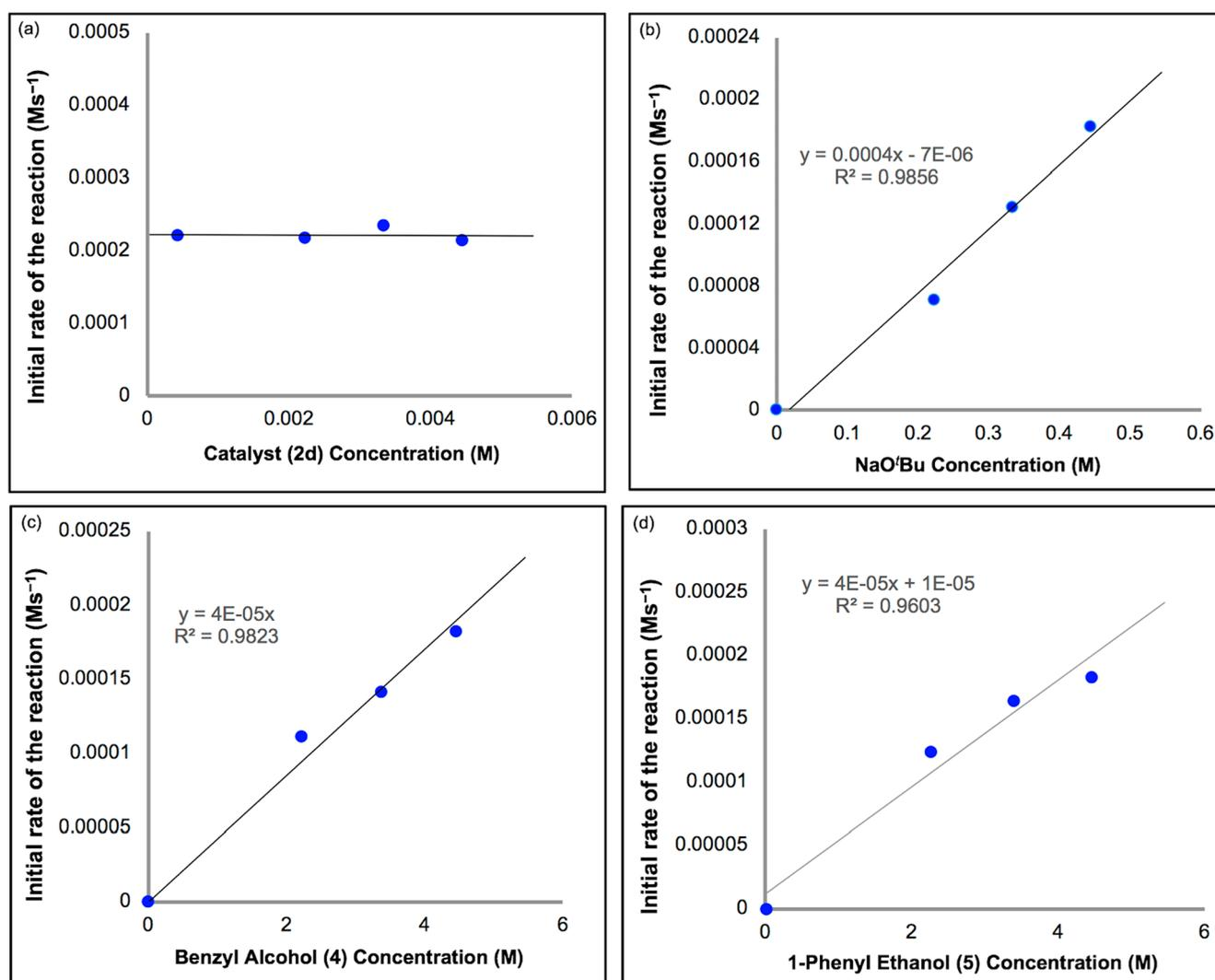
**Figure 6.** Variation of initial rate of Guerbet reaction with concentration of (a) **2d**, (b) NaO'Bu, (c) benzyl alcohol, and (d) 1-phenyl ethanol.
