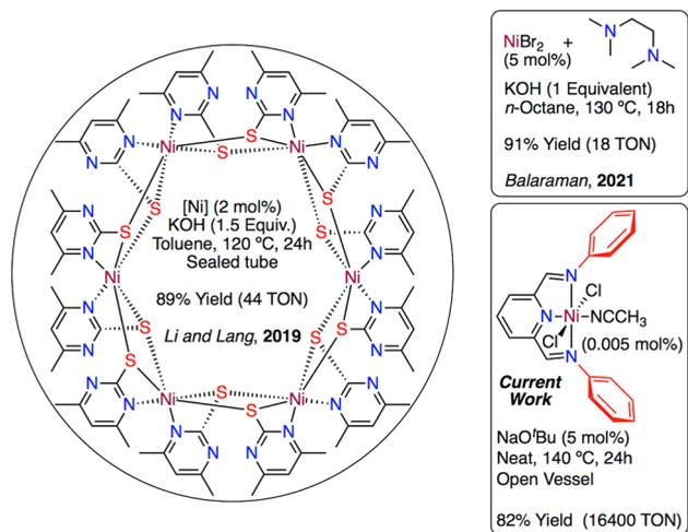
**Figure 1.** Homogeneous Ni catalysts reported for  $\beta$ -alkylation of 1-phenyl ethanol with benzyl alcohol.
