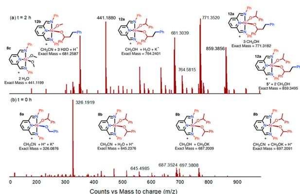
**Figure 5.** HRMS analysis of the reaction mixture containing **4** and **5** in the presence of 0.5 mol % **2d** and 5 mol % Na<sup>t</sup>BuO at  $t = 0$  h at room temperature and at  $t = 2$  h at 140 °C. Also see Figures S80–S94.
