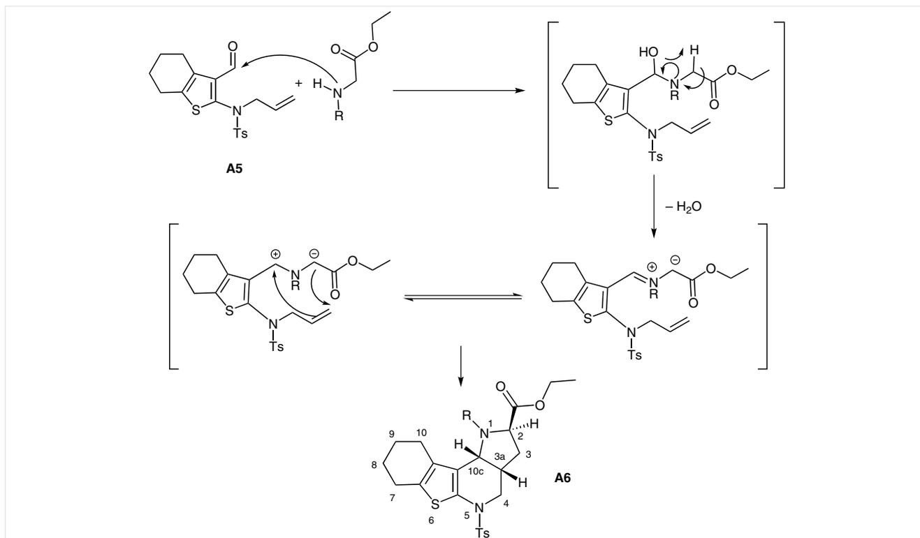
**Scheme 6** Plausible mechanism for the 1,3-dipolar cycloaddition of compound **A5** and N-R substituted 2-amino ethyl acetate **C** (one enantiomer of compound **A6** is depicted).
