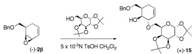
Scheme 6. Reaction of epoxide (–)-2 $\beta$  with 1,2,3,4-di-*O*-isopropylidene- $\alpha$ -*D*-galactopyranose.
