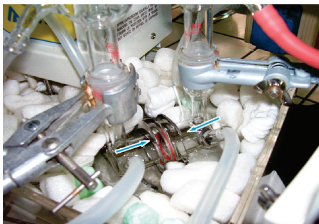
Figure 1. (Top) Biphasic equipment for the membrane allocation. (Bottom) System mounted for the reaction.
