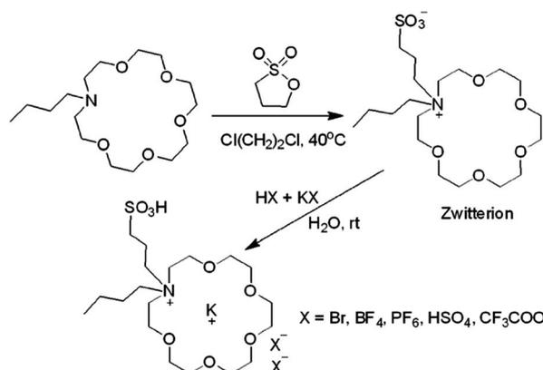
Scheme 2 Synthetic route to Brønsted acidic ionic liquids of *aza*-crown ether complex cations.
