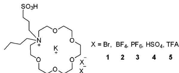
Scheme 1 Structure of Brønsted acidic ionic liquids of *aza*-crown ether complex cations.
