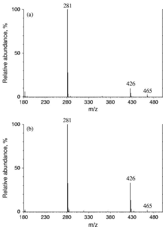
**Figure 1.** Isobutane-Cl mass spectra of (a) **12** and (b) **13**.
