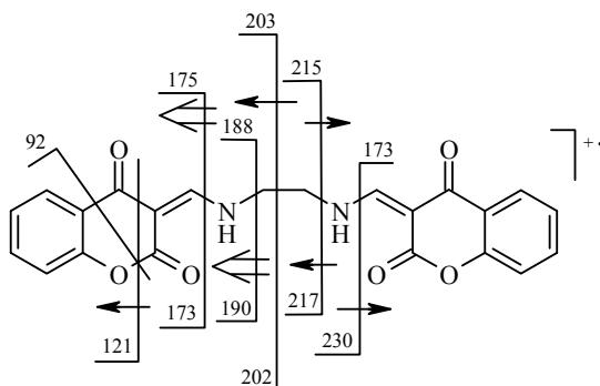
In the mass spectrum of compound **6c**, there was a molecular ion peak at  $m/z$  458. Its dissociation under electron impact is shown in the following scheme.
