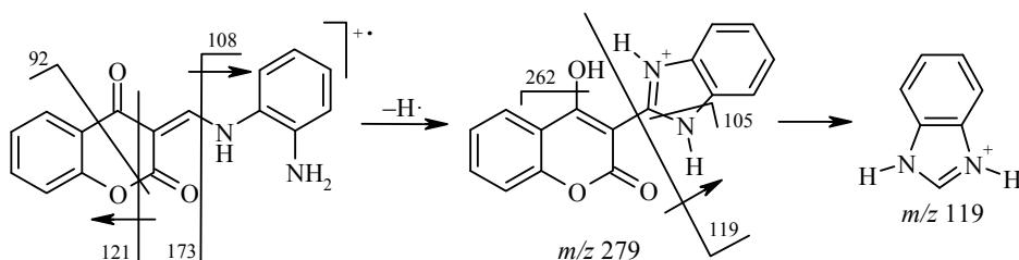
The mass spectrum of compound **6b** contained a molecular ion peak at  $m/z$  404 and also peaks for fragments arising from stepwise cleavage of the bonds as shown below.
