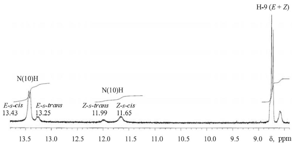
Fig. 1. The downfield part of the  $^1\text{H}$  NMR spectrum of compound **5b**.
