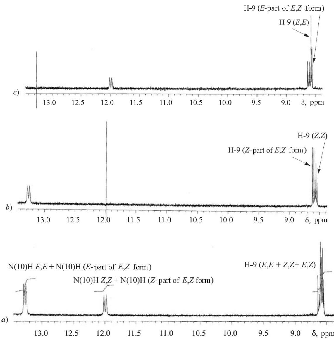
Fig. 2. The downfield part of the  $^1\text{H}$  NMR spectrum of compound **6a**: *a*) The spectrum without spin-spin decoupling from the N(10)H and H-9 protons; *b*) the spectrum with suppression of the N(10)H signals from the Z,Z isomer; *c*) the spectrum with suppression of the N(10)H signals from the E,E isomer.
