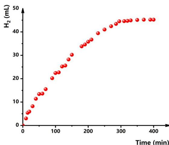
**Figure 2.** Evolution of Dihydrogen Over Time.
