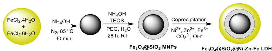
**Scheme 2** Preparation of nanomagnetic  $\text{Fe}_3\text{O}_4@\text{SiO}_2@\text{Ni-Zn-Fe LDH}$
