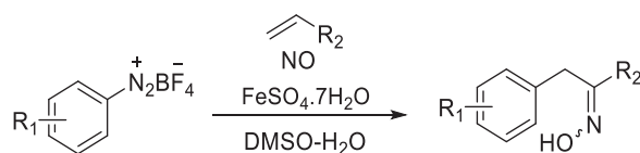
Scheme 1. Formation of oximes by NO gas efflux for recycling NO wastes.
