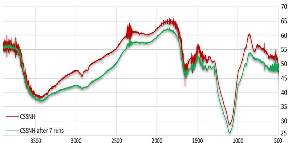
recycled catalyst after seven sequential runs was taken and compared with that of the fresh catalyst (Fig. 3). As can be seen in Fig. 3, no noticeable alteration or change in structure and functionalities of CSSNH is observed and this can be attributed to stability of catalyst.
