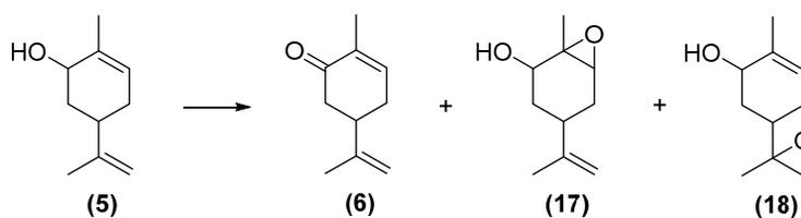
**Scheme 6.** Oxidation of carveol by hydrogen peroxide catalysed by  $M_4(PW_9)_2$  heteropolyanions
