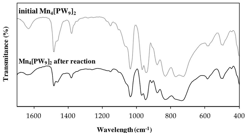
**Fig. 3.** The infrared spectra of the initial  $\text{Mn}_4(\text{PW}_9)_2$  catalyst and the recovered solid after catalysis.
