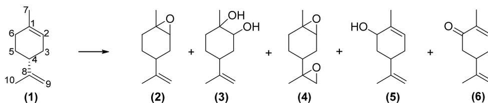
**Scheme 1.** Oxidation of limonene by hydrogen peroxide catalysed by  $\text{M}_4(\text{PW}_9)_2$  heteropolyanions
