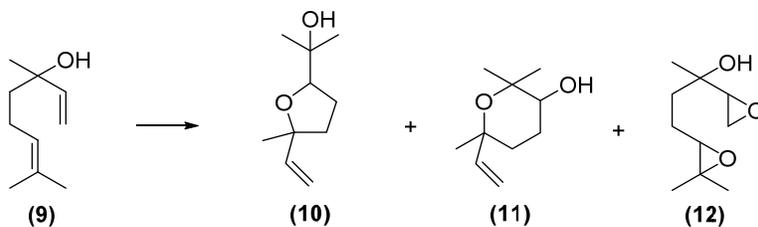
**Scheme 3.** Oxidation of linalool by hydrogen peroxide catalysed by  $\text{M}_4(\text{PW}_9)_2$  heteropolyanions
