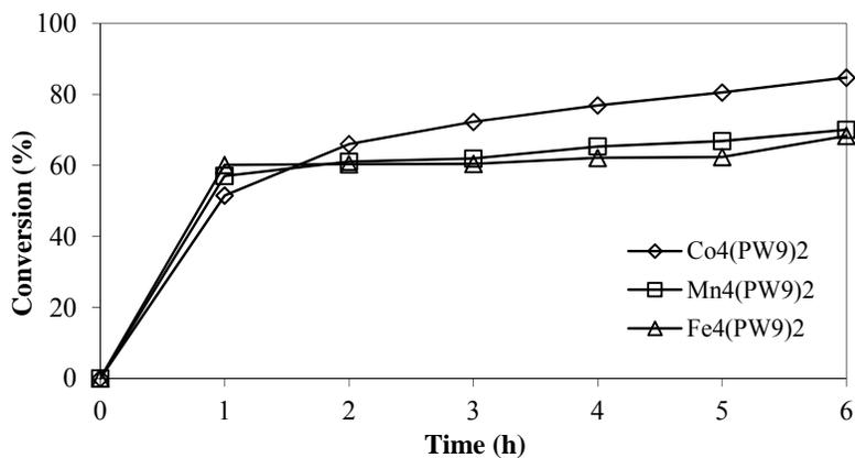
**Fig. 2.** Cyclooctene (3 mmol) oxidation catalysed by sandwich-type POMs (5  $\mu$ mol), with 1.5 mL of CH<sub>3</sub>CN at 80°C and in the presence of H<sub>2</sub>O<sub>2</sub> 30% (3 mmol).
