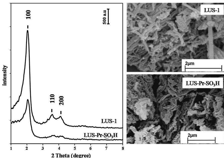
**Fig. 4** X-ray diffraction pattern (*Left*) and SEM images (*Right*) of LUS-1 and LUS-Pr-SO<sub>3</sub>H
