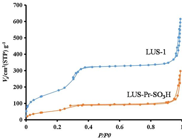
**Fig. 3** Nitrogen adsorption–desorption of LUS-1 and LUS-Pr-SO<sub>3</sub>H
