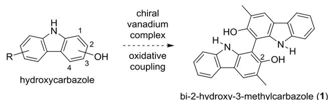
**Scheme 1.** Enantioselective synthesis of bihydroxycarbazoles via chiral vanadium catalyzed coupling of hydroxycarbazoles.
