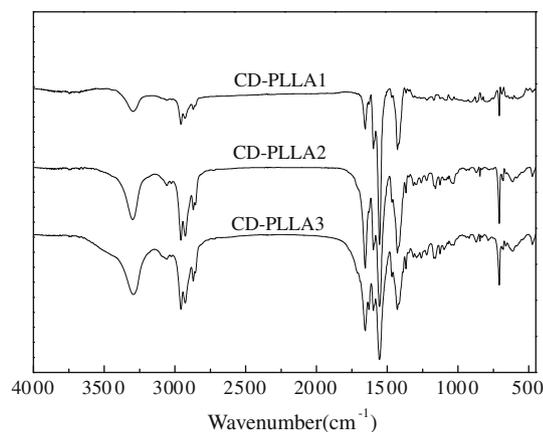
**Fig. 1.** IR spectra of  $\beta$ -CD-PLLA copolymers.
