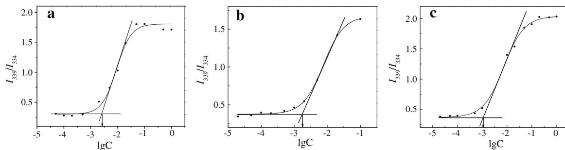
Fig. 5. Plots of  $I_{339}/I_{334}$  versus logarithm of  $\beta$ -CD-PLLA10 (a),  $\beta$ -CD-PLLA30 (b) and  $\beta$ -CD-PLLA50 (c) concentrations.
