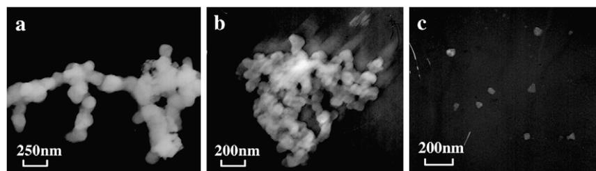
Fig. 7. TEM images of  $\beta$ -CD-PLLA10 (a),  $\beta$ -CD-PLLA30 (b) and  $\beta$ -CD-PLLA50 (c) copolymer micelles.
