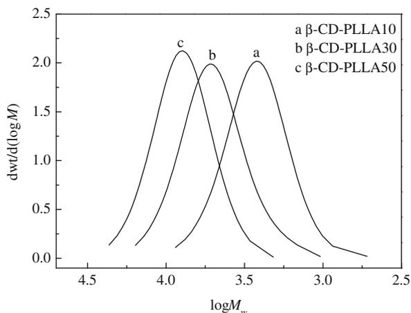
Fig. 3. GPC traces of  $\beta$ -CD-PLLA copolymers.
