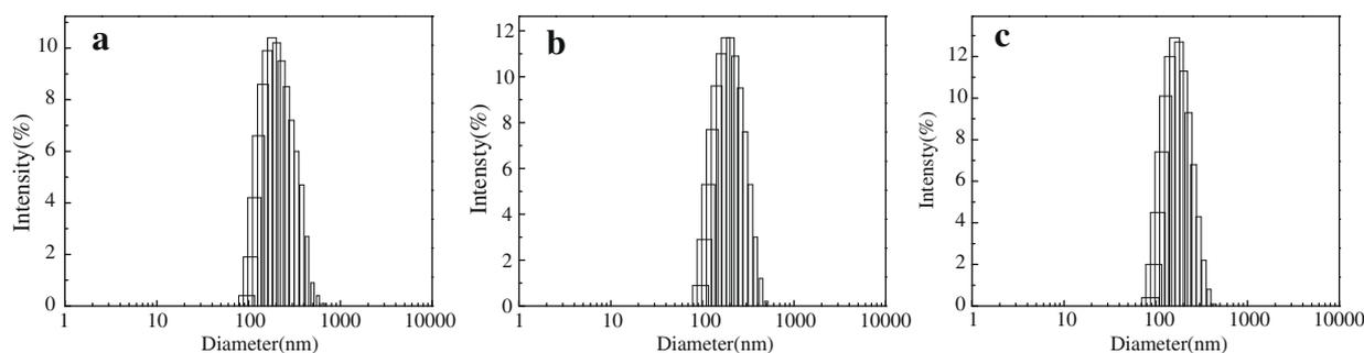
Fig. 6. The size distributions of  $\beta$ -CD-PLLA10 (a),  $\beta$ -CD-PLLA30 (b) and  $\beta$ -CD-PLLA50 (c) copolymer micelles in water measured by DLS.
