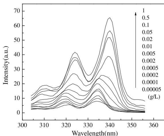
Fig. 4. Excitation spectra of pyrene as a function of  $\beta$ -CD-PLLA10 concentration in water.
