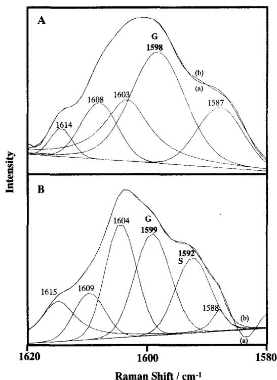
Fig. 3. Component-fitting in the  $\nu(\text{C}=\text{C})$  spectral region. A; *C. japonica* (softwood) and B; *F. crenata* (hardwood). Spectra exhibit (a) experimental data and (b) calculated data from resolved spectra. Number show peak position for each resolved peaks. Proposed guaiacyl- and syringyl-markers are indicated as G and S, respectively. The experimental spectra were obtained with 1  $\text{cm}^{-1}$  resolution, 100 scans, and 200 mW laser using wood meals.
