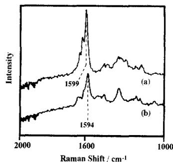
Fig. 2. NIR-FTR spectra of (a) guaiacyl DHP and (b) syringyl DHP, with  $4\text{ cm}^{-1}$  resolution, 200 scans, and 200 mW laser.
