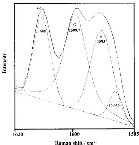
Fig. 6. NIR-FTR spectra of wood block (*K. pictus*) and resolved spectra for component-fitting. Spectra exhibit (a) experimental data and (b) calculated data from resolved spectra. Numbers show peak positions for each resolved peaks. Proposed guaiacyl- and syringyl-makers are indicated as G and S, respectively. The experimental spectra were obtained with  $4\text{ cm}^{-1}$  resolution, 200 scans, and 200 mW laser.
