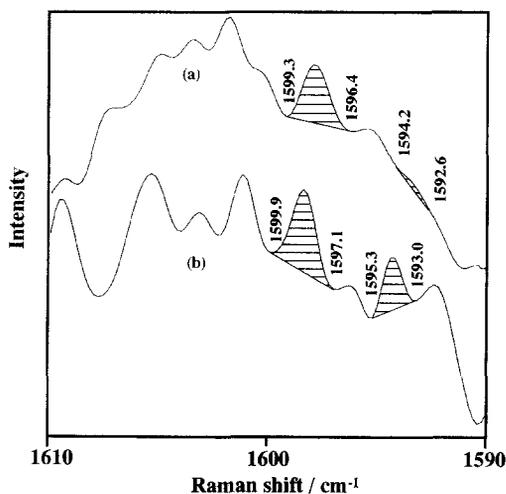
Fig. 4. NIR-FTR spectra of (a) *P. densiflora* (softwood) and (b) *P. strobilacea* (hardwood) in the  $\nu(\text{C}=\text{C})$  region. The spectra were obtained with  $1\text{ cm}^{-1}$  resolution, 100 scans, and 200 mW laser using wood meals. The area strength of the shaded area were utilized to estimate S/G ratio.
