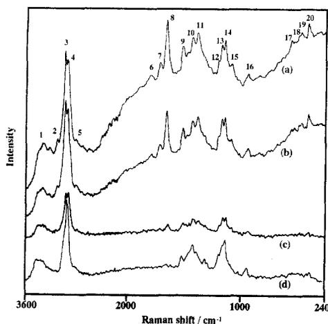
Fig. 1. NIR-FTR spectra of (a) wood meal (untreated), (b) extract-free, (c) holocellulose, (d)  $\alpha$ -cellulose, prepared from *F. crenata*. The spectra were obtained with  $8\text{ cm}^{-1}$  resolution, 200 scans, and 200 mW laser.
