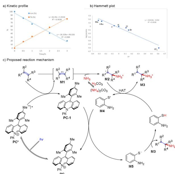
**Figure 5.** Kinetics investigations and proposed mechanism for the reaction.
