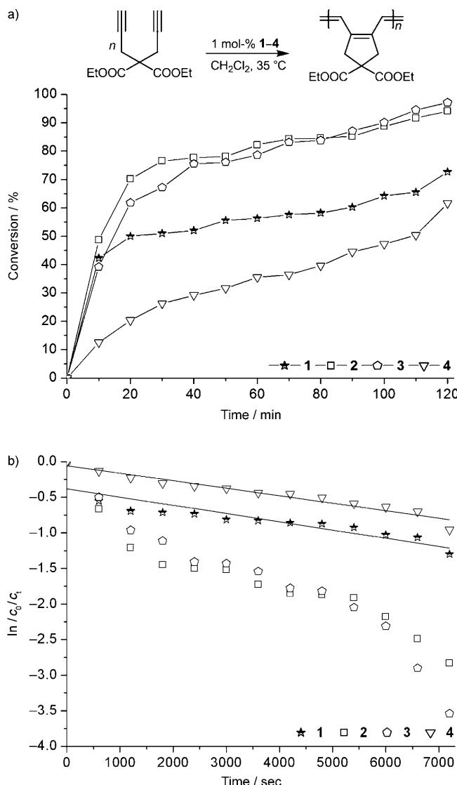
Figure 6. Kinetics of the cyclopolymerization of DEDPM by the action of 1–4. a) conversion versus time, b) First order plot. [initiator]=4.2 mM, [DEDPM]=0.42 M.
