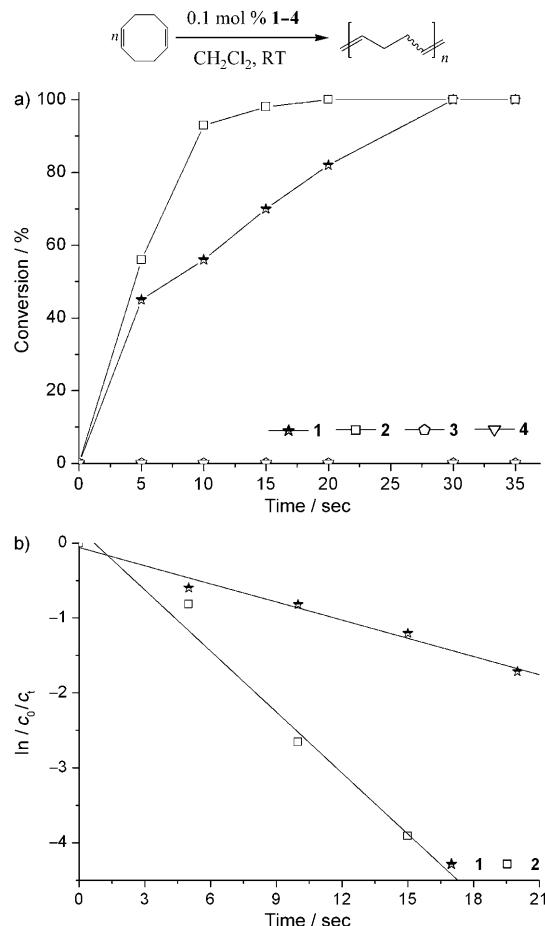
Figure 2. a) Kinetics of ROMP of COD by the action of **1–4**. b) First-order plots for **1** and **2** in the ROMP of COD. [initiator]=1.8 mM, [COD]=1.8 M.
