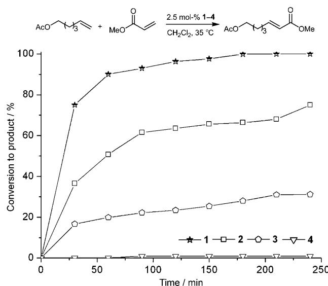
Figure 4. CM of methyl acrylate with 5-hexenyl acetate by the action of **1–4**. [initiator] = 4.3 mM, [5-hexenyl acetate] = [methyl acrylate] = 0.18 M.
