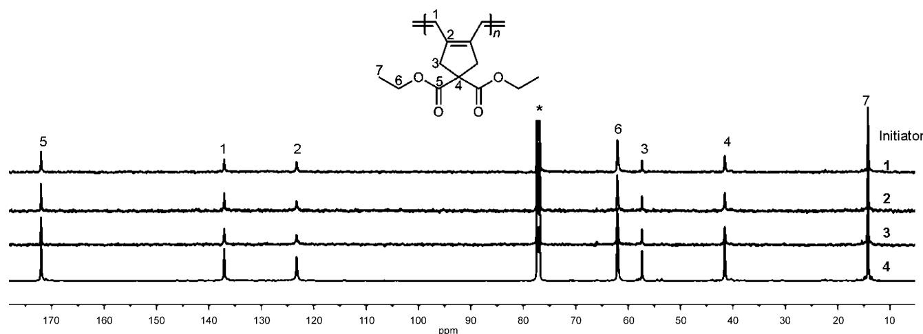
Figure 5.  $^{13}\text{C}$  NMR spectra of poly(DEDPM) in  $\text{CDCl}_3$ ; (\*) denotes  $\text{CDCl}_3$ .
