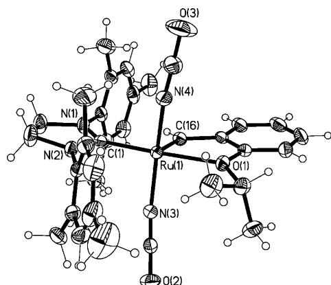
Figure 1. X-ray structure of **1**. Selected bond lengths (pm): Ru(1)-C(16), 180.8(4); Ru(1)-C(1) 196.7(3); Ru(1)-N(3) 202.2(4); Ru(1)-N(4) 200.8(4); Ru(1)-O(1) 225.6(2). Selected bond angles (°): C(16)-Ru(1)-N(4) 96.55(16); C(16)-Ru(1)-N(3) 100.47(16); C(16)-Ru(1)-C(1), 101.75(16); C(1)-Ru(1)-N(4), 91.84(14); C(1)-Ru(1)-N(3), 93.56(13); N(4)-Ru(1)-N(3), 160.68(14); C(16)-Ru(1)-O(1), 79.38(14); C(1)-Ru(1)-O(1), 177.30(12); N(4)-Ru(1)-O(1), 85.59(11); N(3)-Ru(1)-O(1), 88.62(11).
