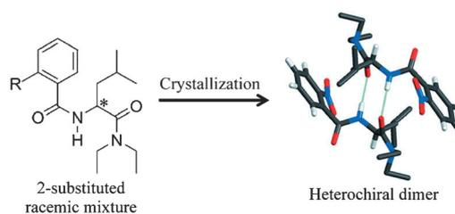
Scheme 1. 2-substituted benzoyl leucine diethyl amides form heterochiral dimers with two hydrogen bonds (shown as cyan lines) in the solid state.
