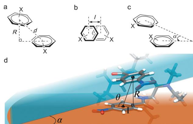
Figure 2. Geometric parameters used to define the orientation of two interacting aromatic rings. a) The distance  $R$  of the ring centroid to the plane defined by the opposite ring, and the ring-centroid-to-ring-centroid distance ( $d$ ). b) The horizontal displacement  $I$  between two ring centroids. c) The tilt angle  $\alpha$ . d) The displacement angle  $\theta$  is defined by the smaller of the two angles defined by the ring-to-ring centroids to the plane of the benzoyl rings.
