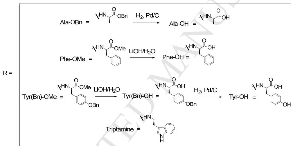
**Scheme 1.** Synthesis of dendrimers **4-11** by the divergent approach. *Reagents and conditions:* (i) HOOCH, 40°C, 48 h, (ii) HATU/DIPEA (iii) H<sub>2</sub>, Pd/C (iv) LiOH.H<sub>2</sub>O
