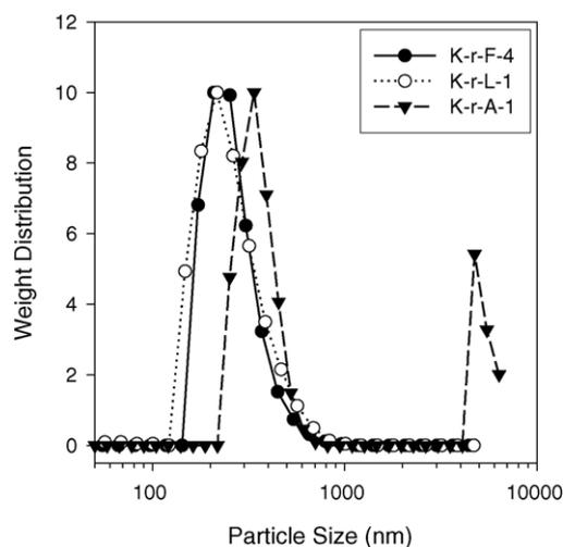
Fig. 3. Size distribution curves of drug particles measured by quasi-elastic light scattering method.
