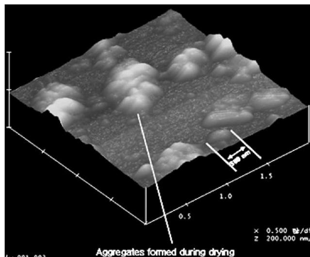
Fig. 5. Atomic force micrograph of drug nanoparticles prepared with using amino acid copolymers (K-b-F-1).
