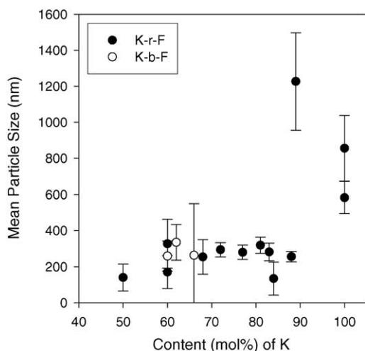
Fig. 4. Mean particle sizes of drug nanocrystals vs. K content in copolymers. The nanocrystals were prepared in the presence of amino acid copolymers of various K contents.
