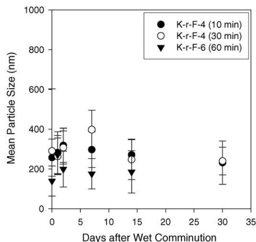
Fig. 7. Plot of mean particle size vs. time shows the physical stability of drug nanosuspensions at room temperature after wet comminution. Wet comminution times are given in parentheses.
