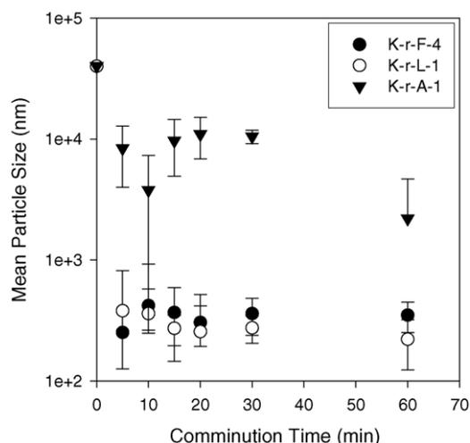
Fig. 2. Mean particle size changes of various copolymer systems as a function of comminution time.
