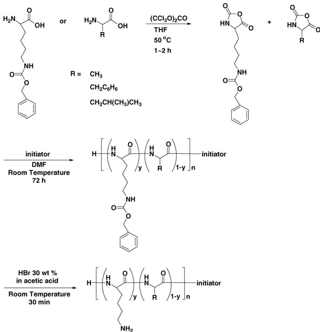
Fig. 1. Reaction schemes of amino acid copolymers.
