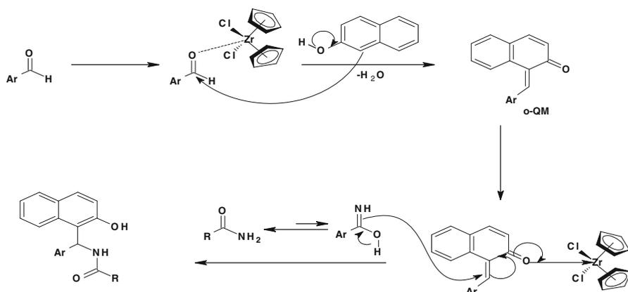
**Scheme 2** Proposed mechanism for the synthesis of 1-amidoalkyl-2-naphthols using  $\text{Cp}_2\text{ZrCl}_2$
