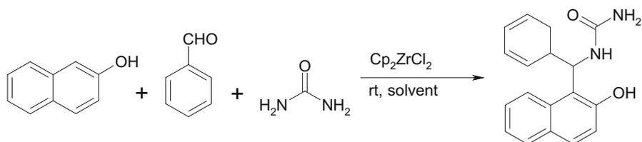
**Scheme 1**  $\text{Cp}_2\text{ZrCl}_2$  catalyzed multi-component synthesis of 1-amidoalkyl-2-naphthols
