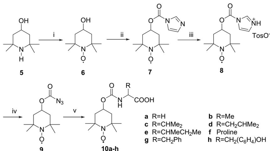
Scheme 1. Reagents and conditions: (i) Na<sub>2</sub>WO<sub>4</sub>/H<sub>2</sub>O<sub>2</sub>/EDTA; (ii) *N,N'*-carbonyldiimidazole/THF; (iii) *p*-toluenesulfonic acid monohydrate; (iv) NaN<sub>3</sub>/water, stir; (v) amino acids/MgO, stir, 24 h.
